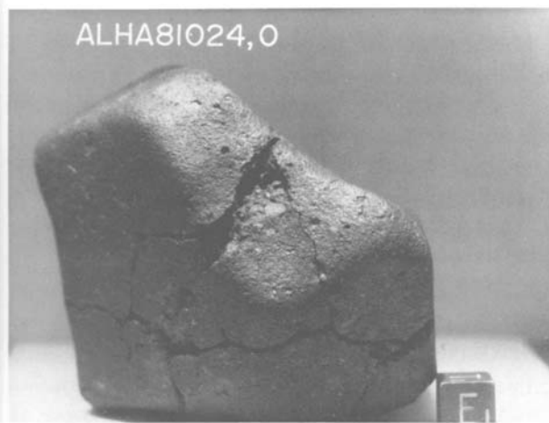
FIGURE 23.—ALHA81024, L3 chondrite, a rounded angular stone with several deep fractures, with a reddish brown weathered surface.
