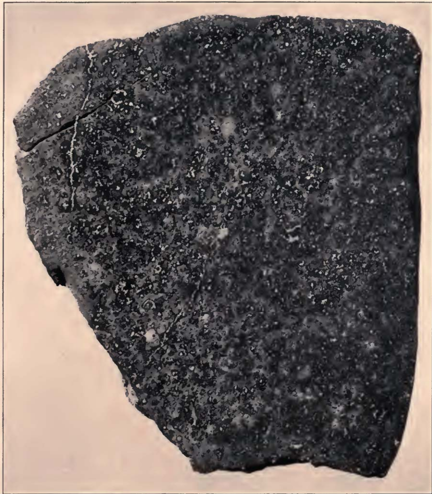
Section of Shelburne meteorite, showing metallic veins and distribution of metallic grains, \times \frac{1}{3} .
