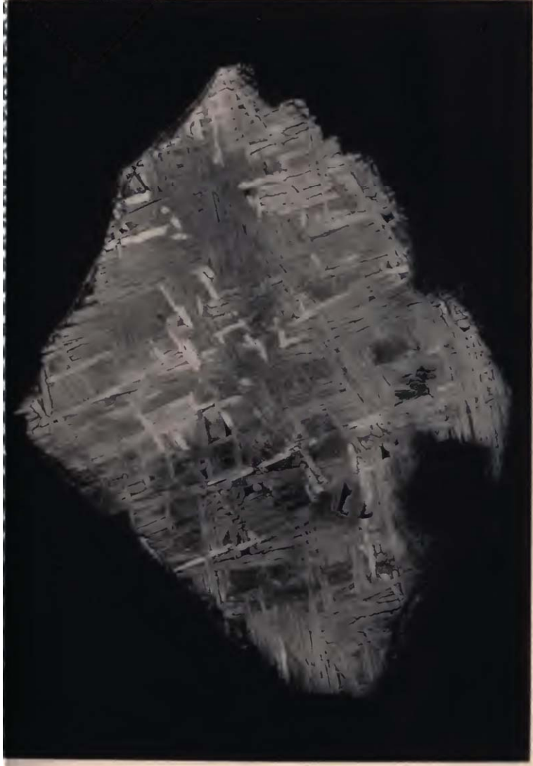
ETCHED SECTION OF THE SHREWSBURY IRON METEORITE. SHOWING WIDMANSTÄTTEN FIGURES.
